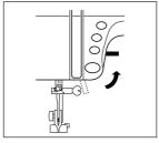
Raise the presser foot. Press the Up/Down needle button to raise the thread take-up lever to its highest position.
