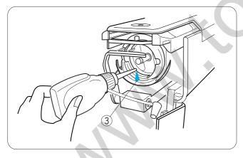
Open the hook cover and remove the bobbin case. Clean the inside of the hook with the lint brush.
