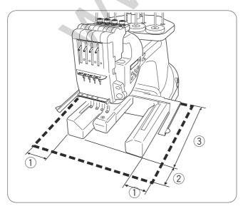
Provide a sufficient space around the machine to allow the hoop to move freely.
