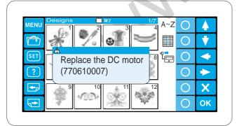
When the total running time of the DC motor reaches 1,000 hours, a message will appear advising you to replace the DC motor.
