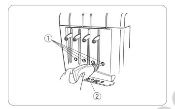
Apply a few drops of oil to the needle bar through the holes in the front cover.
