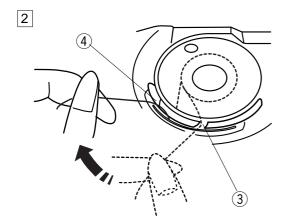
2 Guide the thread into the notch on the front of the bobbin holder.
