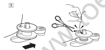
3 Push the spindle to the right. Press the start/stop button while holding the end of the thread. Stop the machine after the bobbin is wound a few layers. Cut the thread close to the hole in the bobbin.
