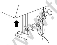
Release the threader knob slowly while holding the thread end with your hand. A loop of the thread is pulled up through the needle eye.
