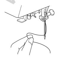
Remove the loop from the threader and pull out the thread end from the needle eye.
