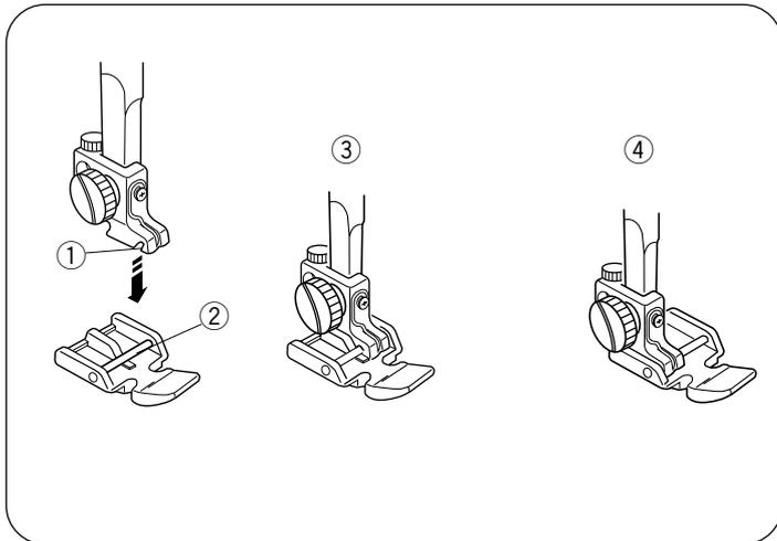
To sew on the left side of the zipper, attach the foot holder to the right pin on the zipper foot.
