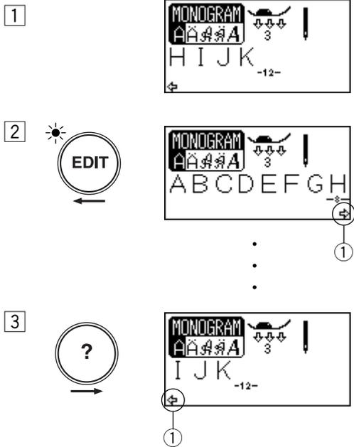
1 The LCD screen only shows 8 characters of a monogram at a time. If the entire text is not displayed, press the edit key or help key to scroll the text.
