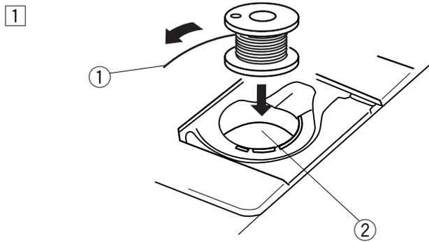
1 Place the bobbin in the bobbin holder with the thread running off counterclockwise.
