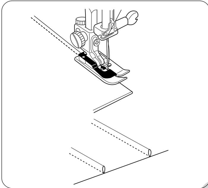
Fold a fabric with the right side together. Place the folded fabric under the blind hem foot. Align the edge of the fold with the guide on the foot, and lower the foot. Sew while guiding the edge of the fold along the guide. Open the fabric and press the tuck to one side.
