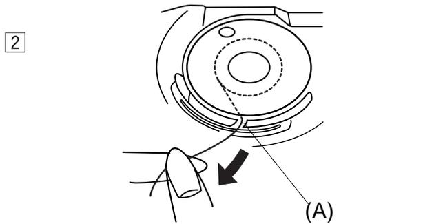
2 Guide the thread into notch (A) on the front of the bobbin holder.
