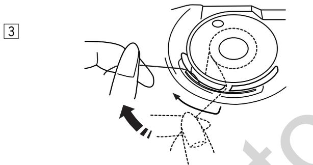
3 Draw the thread to the left, sliding it between the tension spring blades.
