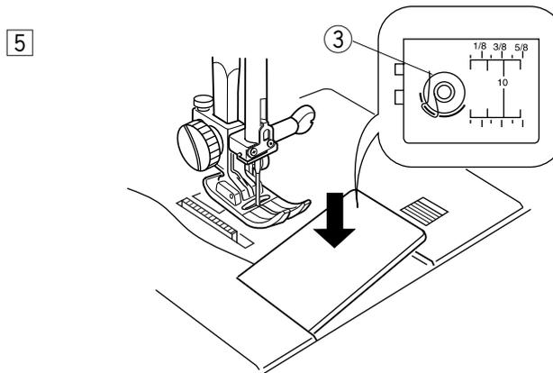
5 Pull out about 10 cm (4") of thread to the rear. Refer to the threading chart shown on the hook cover plate. Attach the hook cover plate.
