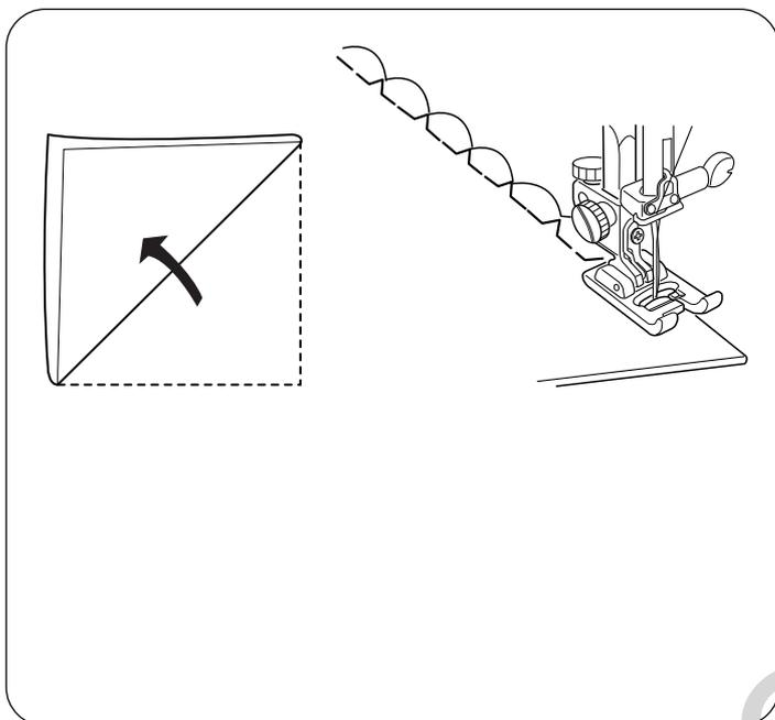
Use a light weight fabric (tricot, for example). Fold the fabric as shown and stitch on the fold. Allow the needle to just clear the folded edge to create a shelled edge. You may need to increase the needle thread tension slightly.
