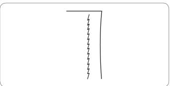
This is a narrow stretch stitch designed to eliminate puckering on knit fabrics and bias seams, while permitting the seam to be pressed completely open at.
