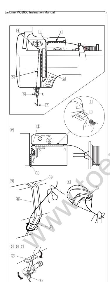
Threading the Machine Janome Quilting & Sewing Machine Raise the presser foot lifter to raise the presser foot.
