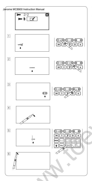
**Touch panel calibration** Janome Quilting & Sewing Machine If the touch panel keys seem out of alignment, calibrate the key position as follows.
