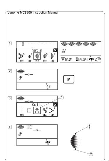
**Programming Auto-lock State** Programming patterns 147 and auto-lock stitch. The machine will sew the pattern, auto-lock stitch, and stop automatically.
