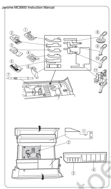
Accessories Storage Janome Quilting & Sewing Machine The accessories can be conveniently stored in the foot storage compartment under the top cover and in the extension table.
