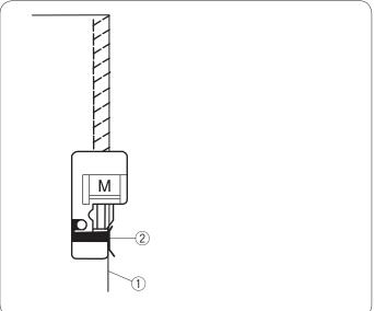
This stitch is recommended for sewing such fabrics as synthetic knits and stretch velour as it provides the greatest amount of elasticity and strength.
