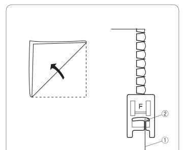
Use a light weight fabric (tricot, for example). Fold the fabric as shown and stitch on the fold.
