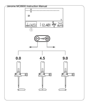
Adjusting the needle drop position Quilting & Sewing Machine
