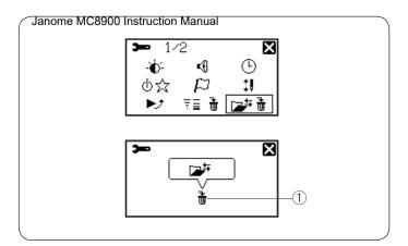
Deleting stored pattern combination & Sewing Machine All the pattern combinations stored in the memory bank can be deleted at one time.
