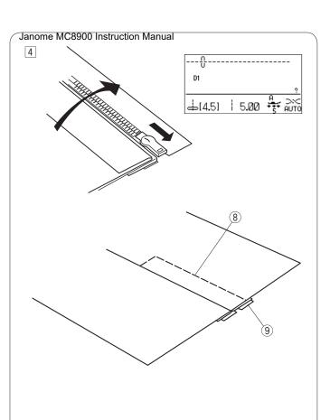
4 Close the zipper and spread the fabric open at with the right side facing up.
