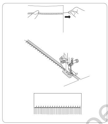
Fringing adds a special touch on table linens and shawls. Choose a rm, woven fabric like linen where threads can be removed easily.
