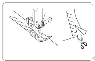
This stitch is ideal for finishing edges of stretch fabrics. It seams and finishes the fabric edges simultaneously.
