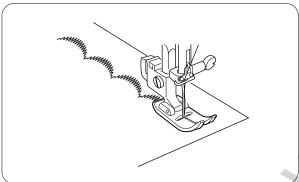
Determine the appropriate stitch density by test sewing.
