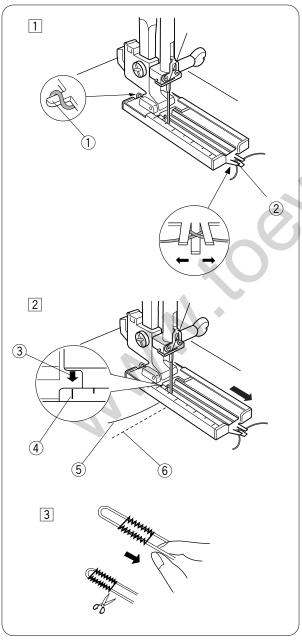
With the buttonhole foot raised, hook the filler cord on the spur at the back of the foot.
