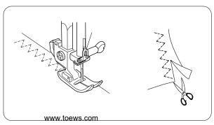
This stitch is used to finish a raw edge on synthetics and other fabrics that tend to pucker. Place the fabric to leave a 5/8" (1.6 cm) allowance.
